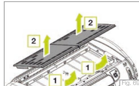
6. Using a screwdriver, remove the fixing screws of the upper panel as shown in the figure.
