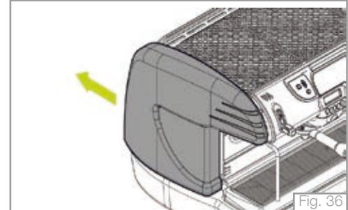
4. Pull the side panel away from the machine and remove it as shown in the figure.
