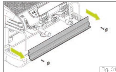
3. Remove the plate covering the system by loosening the two fastening screws.
