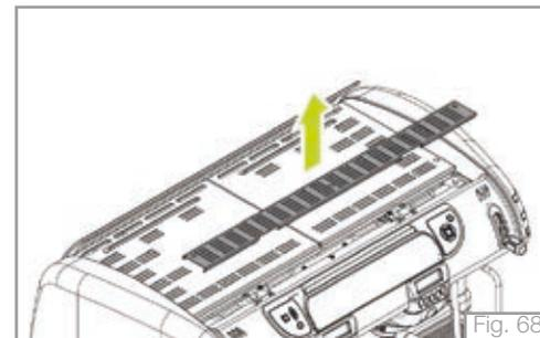
5. Using the rear part as the fulcrum, pull up the rear plates of the cup warmer plate and remove them as shown in the figure.
