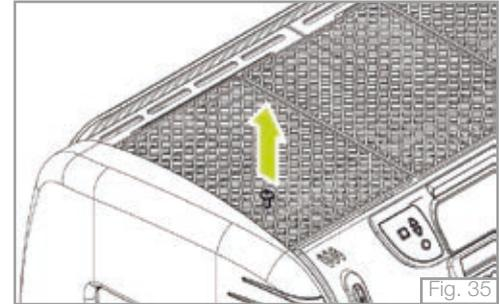
3. Slide the side panels towards the rear of the machine until they stop.
