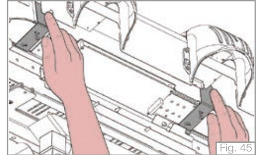
4. Extract the control panel upwards as shown in the figure.
