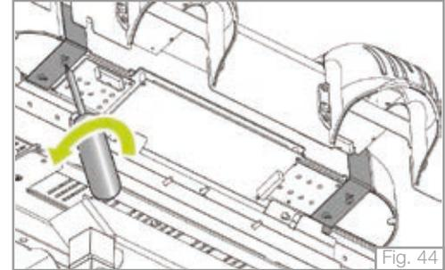
3. Press the two fixing brackets of the control panel as shown in the figure.
