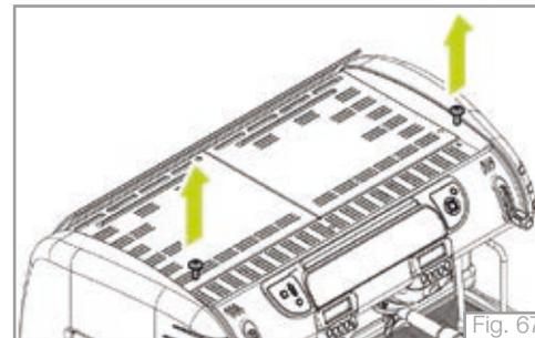
4. Remove the front plate of the cup warmer plate as shown in the figure.
